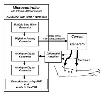
Fig. 1. The developed device for detection of acupuncture point
