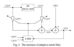
The adaptive system between the input x(n) and the output e(n) is an adaptive notch filter, which forms several notch filters centered at frequency of the sinusoidal components.
